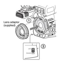
① Align the alignment pin of the lens adaptor with the recess at the top of the
